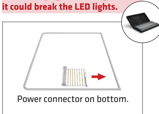
**Step 3:** Attach each LED Light Array to top and bottom of frame.
