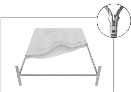
**Step 5:** Zip the edge of graphic beyond the center point as shown to hold the center pole in place. Zip the remaining side and bottom to meet at the corner.
