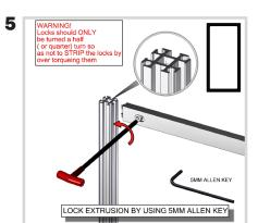
Using the 5mm Allen-T attach your supporting PH1 extrusions to the small PX extrusions.
