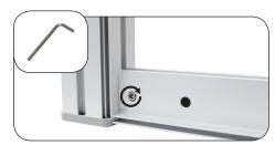
**3.** Tighten Socket Screw with allen wrench to secure.
