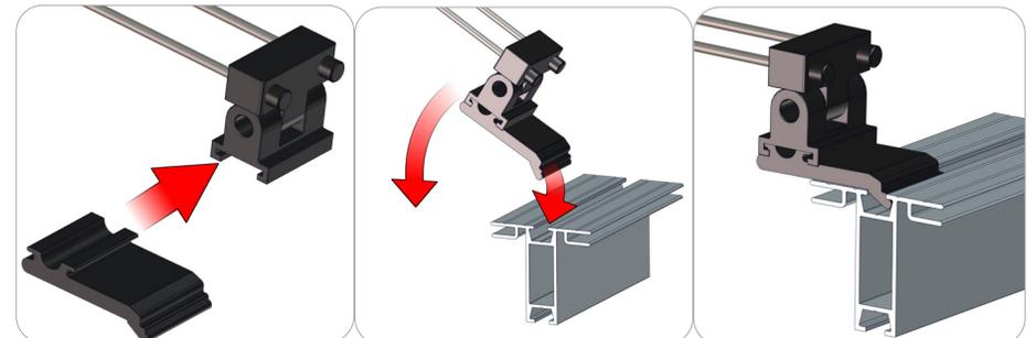
First, slide the light clip into the dove tail end of the spot light. Second, rest the light clip into the extrusion channel. Make adjustments to the spot light if necessary.
