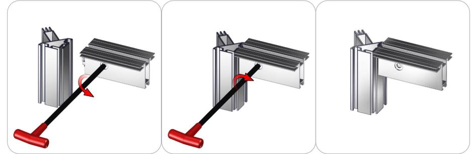
First, with the cam lock disengaged, place the cam lock teeth into the extrusion channel. Second, use the allen key tool to lock it in place. Make half turns clock-wise to engage the cam lock. Do not over tighten the lock buttons.
