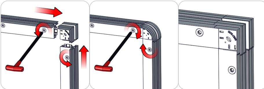
First, make sure the cam lock button is unlocked. Second, insert the cam lock teeth in to corner bracket channel. Third, tighten the cam lock button. Use the allen key tool to turn the lock buttons, make quarter turns and do not over tighten the lock buttons. Repeat for opposite end.
