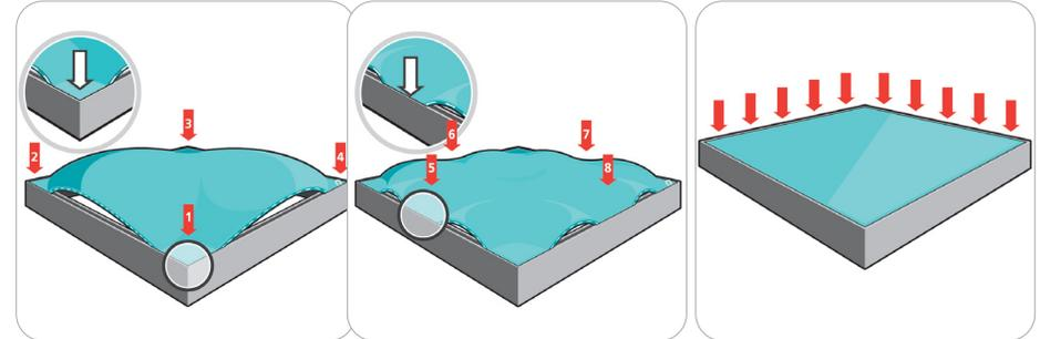
First, insert the silicone edge frame corners into the frame graphic channel (points 1 through 4). Second, insert the silicone edge frame sides into the frame graphic channel (points 5 through 8). Third, push the remaining silicone edge fabric into the frame graphic channel. Similar setup is recommended for the opaque liner. To remove these panels, simply pull the loop tag sewn near a corner.
