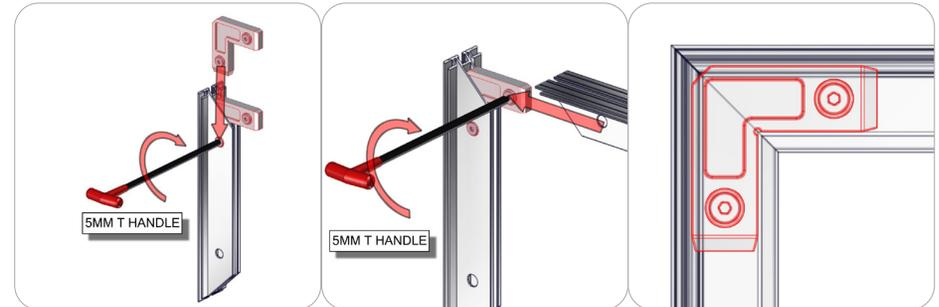
First, insert the corner connector into the extrusion while holding in the lock button. Then, slide the next extrusion onto the same corner connector again holding in the lock button. Finally, use the provided allen key to lock the corner connector in place. Use the allen key tool to press the lock buttons, make quarter turns and do not over tighten the lock buttons.
