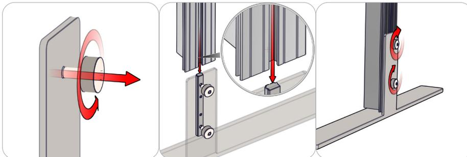
First, loosen the thumb screws and channel bars on the stabilizing bases. Do not disassemble them. Second, slide channel bars into the frame channel flush with the base of the frame. Finally, tighten the thumb screws and channel bars securing the attachment.
