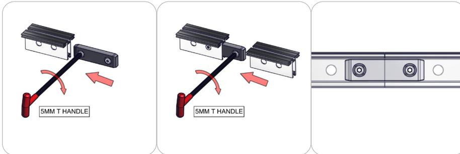
First, insert the in-line connector into the extrusion while holding in the lock button. Then, slide the next extrusion onto the same in-line connector again holding in the lock button. Finally, use the provided allen key to lock the in-line connector in place. Use the allen key tool to turn the lock buttons, make quarter turns and do not over tighten the lock buttons.
