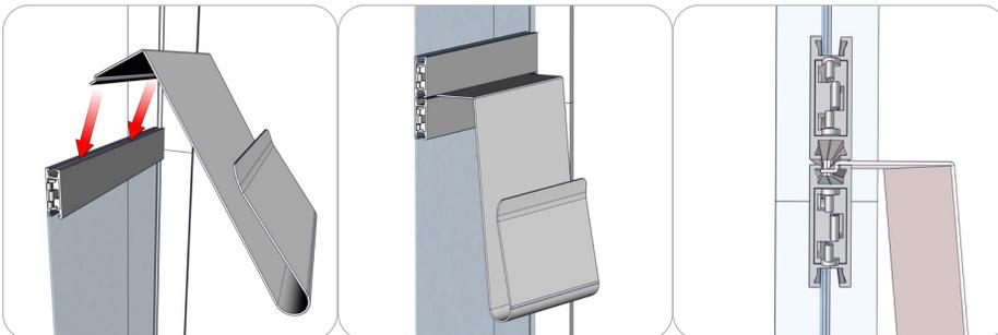
First, have a PH series profile or smaller extrusion with its channel facing up; lock it in place to hold the literature pocket. Second, rest the literature pocket flange into the extrusion top channel. Third, your kit may feature a second extrusion to lock right above the literature pocket.
