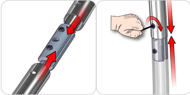
Compress the unlocked connector and slide one tube onto each end. Lock both screws carefully using your hex key tool. Be sure to lock securely, but do not overtighten.
