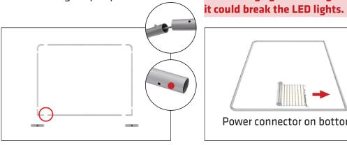
Step 2: Take out the LED Lights and gently unroll on the ground with lights face down. WARNING! Do not drag lights across ground or
